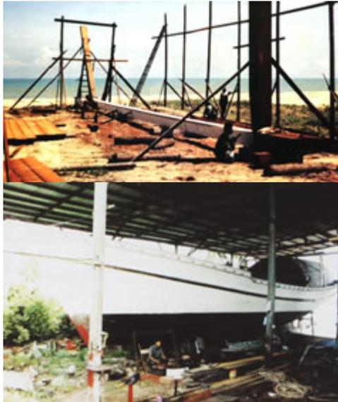
The first step was laying the keel, the length determining the final size of the boat. The keel was then grooved for the first plank with holes drilled at 20cm intervals to take the dowels that held the first plank in place. The position of these holes was marked with a pencil on the edge of the plank to be fixed. The corresponding holes could then be bored in the correct position.
